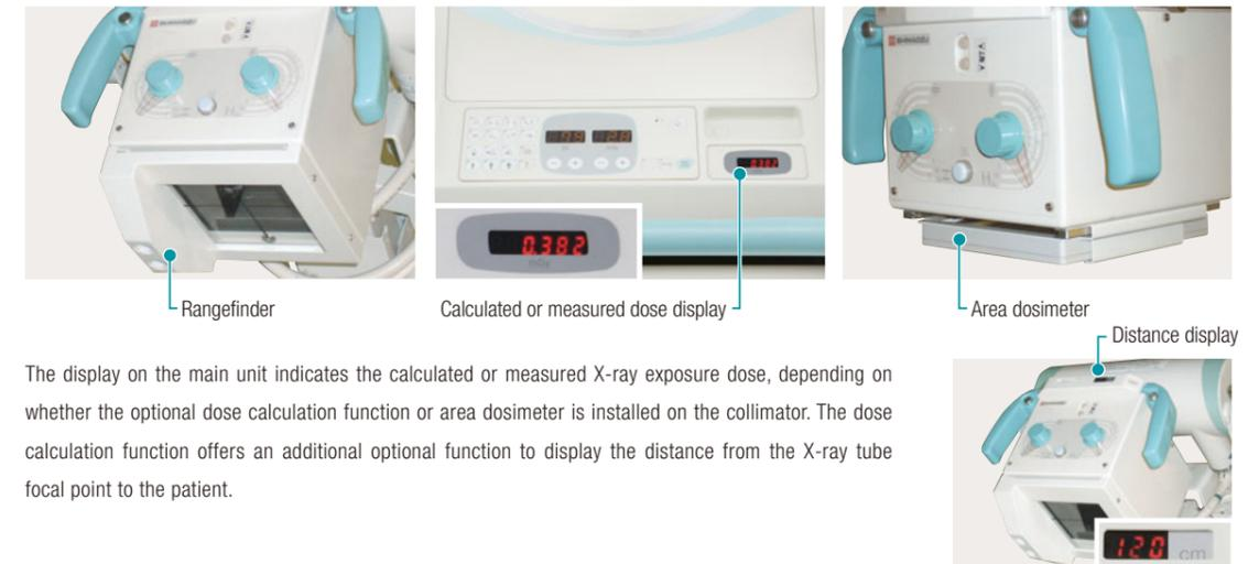
The display on the main unit indicates the calculated or measured X-ray exposure dose, depending on whether the optional dose calculation function or area dosimeter is installed on the collimator. The dose calculation function offers an additional optional function to display the distance from the X-ray tube focal point to the patient.
