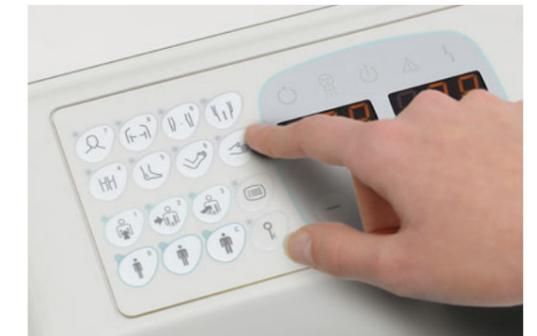
Simply select one of the 72 preset anatomical programs (APR) to configure the optimal radiography conditions for the corresponding radiography region, direction, and body thickness. The focal spot size can also be preset in the high-power type. The collimator efficiently eliminates X-rays outside of the focal spot, creating sharper images.
